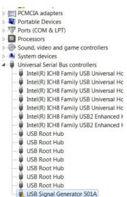
Installing 64-Bit Drivers for the USB Signal Generator
